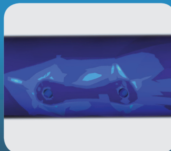
Mini TightRope® Single hole plate showing non-uniform load dispersion with high strain points
