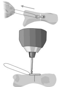
Snap-off shaft from screw and use hand held screw driver to adjust screw position if necessary. Remove suture from final construct and discard. Intra-operative fluoroscopy is recommended to confirm final device placement.
